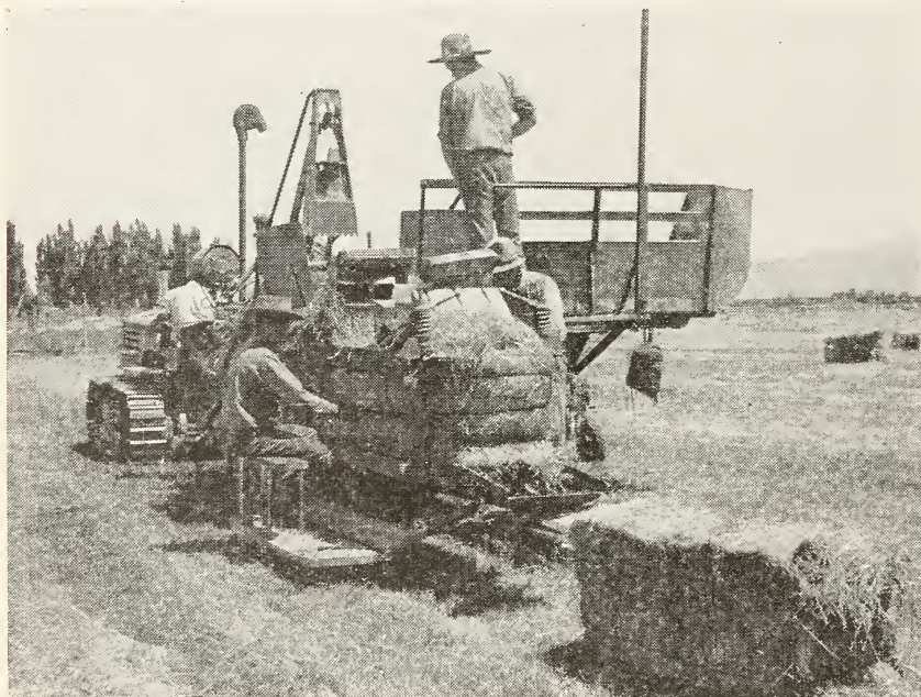
FIGURE 14.—A 3-wire high-capacity type of pickup baler commonly used for baling hay in the West, especially in irrigated regions. The bales produced by these balers weigh more than 125 pounds each.
